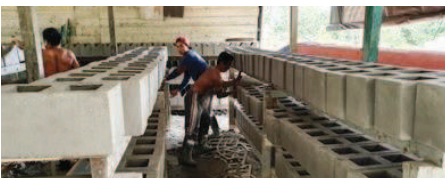
Making over 300 of our own concrete blocks each day
